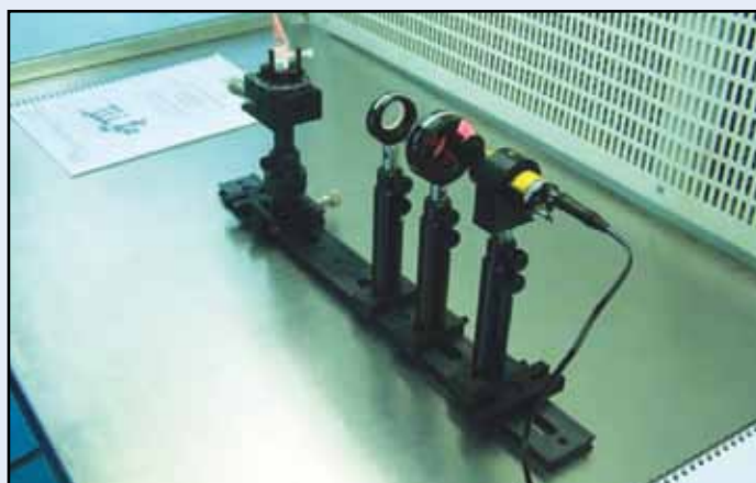
Integrated Optical Wave Guide Characterization Setup (Prism Coupling Technique)
